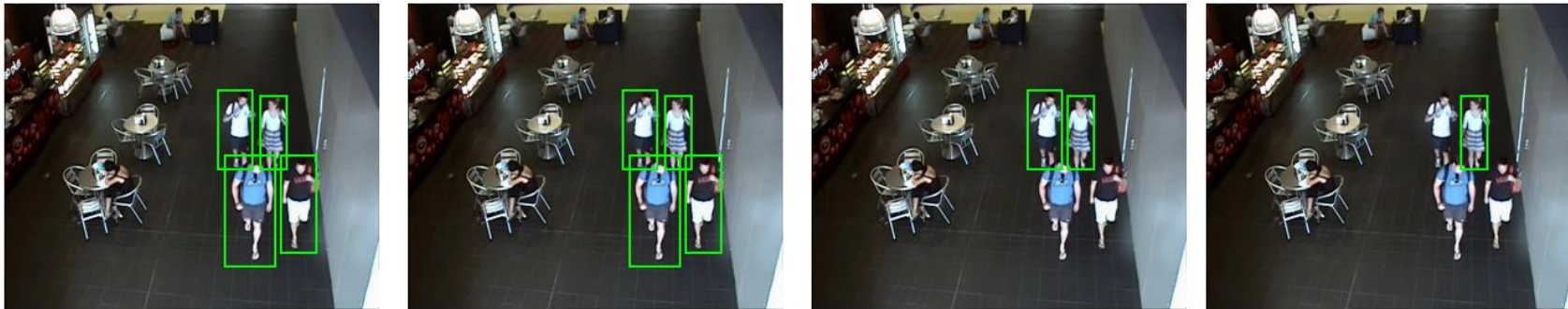
Person retrieved using height, torso, leg and gender module filter
